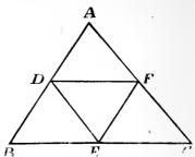
Bisect the sides of the triangle ABC in D, E and F. The weight of each side may be supposed to be collected at its middle point, it is also proportional to the side, and therefore proportional to the opposite side of the triangle DEF; hence the problem becomes the same as the one just solved.
